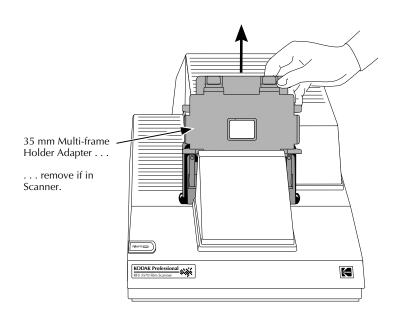
2. If the single-frame holder adapter is not in the Scanner, put it in place in the Scanner.
